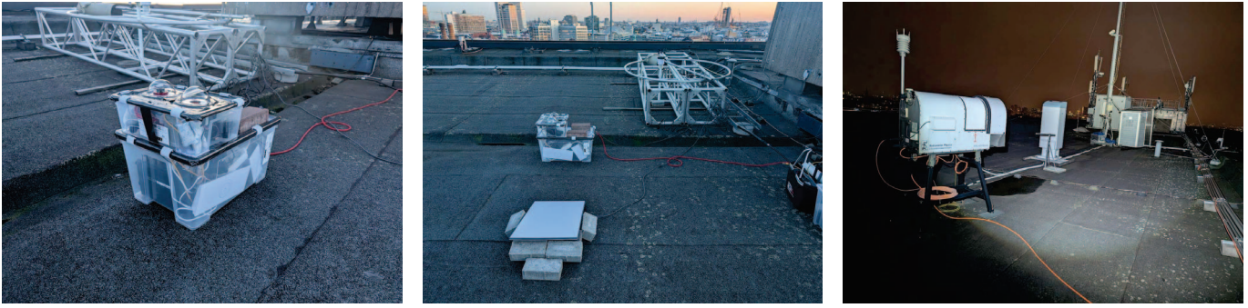
Fig. 1: Left : Close-up photo of stacked transparent plastic boxes containing Starlink measurement equipment on a rooftop. Center : Wide rooftop view showing the Starlink terminal, the stacked box setup, and a nearby weather station. Right : Nighttime image of the rooftop showing the microwave radiometer (left) and the ceilometer (right).
