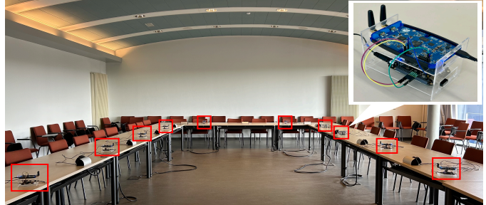
Fig. 3. Indoor deployment of 10 nodes with quasi-grid topology
