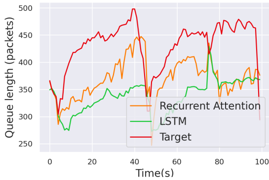
(b) Estimation of the bottleneck load (with emulation) using LSTM and Attention architectures.
