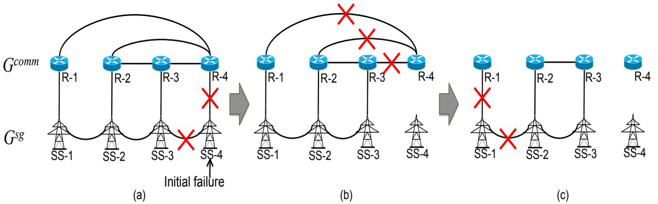
Fig. 1: (Color Online) An illustration of a cascading failure suffered by an interdependent system of size  $N^{sg} = N^{com} = N = 4$  triggered by a failure at node SS-4<sup>3</sup>.
