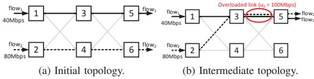
Fig. 3. SDN topology reconfiguration with an overloaded link.
