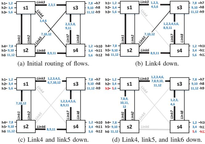
Fig. 4. Network topology and flow routing in the single domain experimental scenario. Switches are connected to the same Floodlight controller and are controlled by one *OptimalFlow* controller (not shown in figure).
