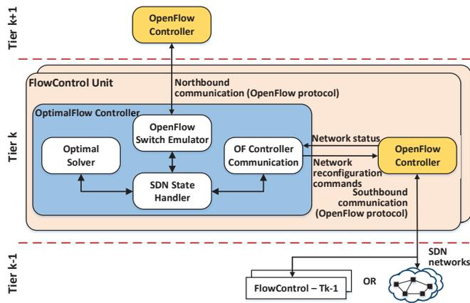
Fig. 2. Detailed architecture of the FlowControl unit.
