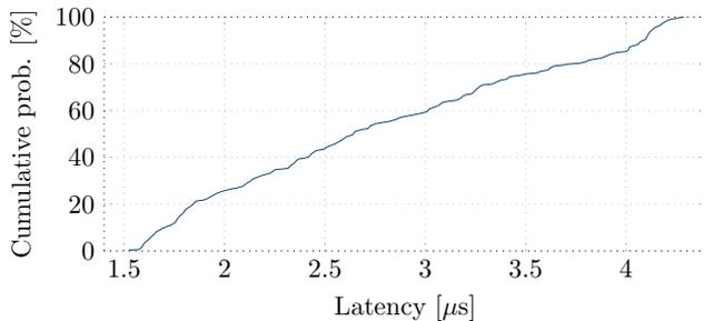
Figure 9. Latency incurred by an OpenFlow meter
