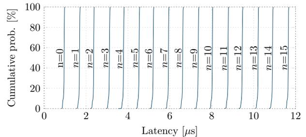
Figure 6. Latency distributions traffic forwarded through the switch  $n$  times
