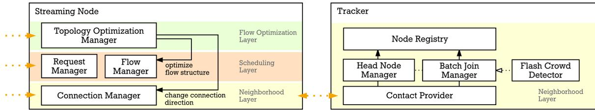
Fig. 2. Extended design, including the core components of the streaming node and tracker as well as their relations.
