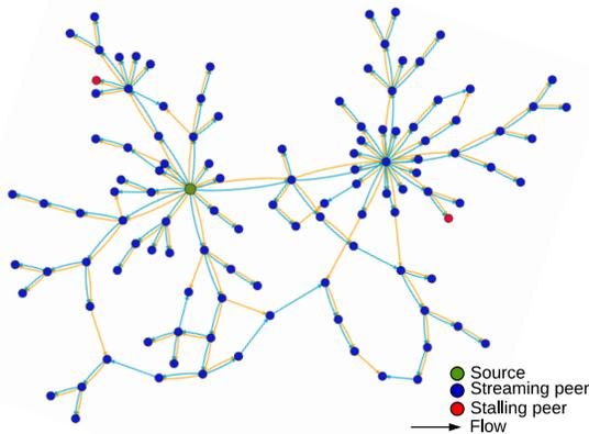
Fig. 3. Example topology for two flows as established by TRANSIT.
