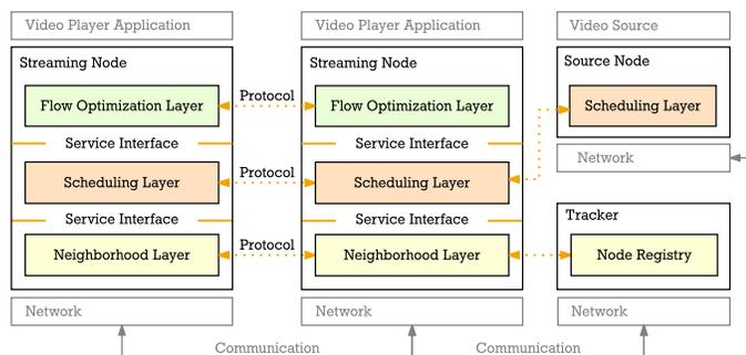
Fig. 1. Conceptual layers of TRANSIT, including the new *Flow Optimization Layer* added by TOPT and introduced in Section IV.
