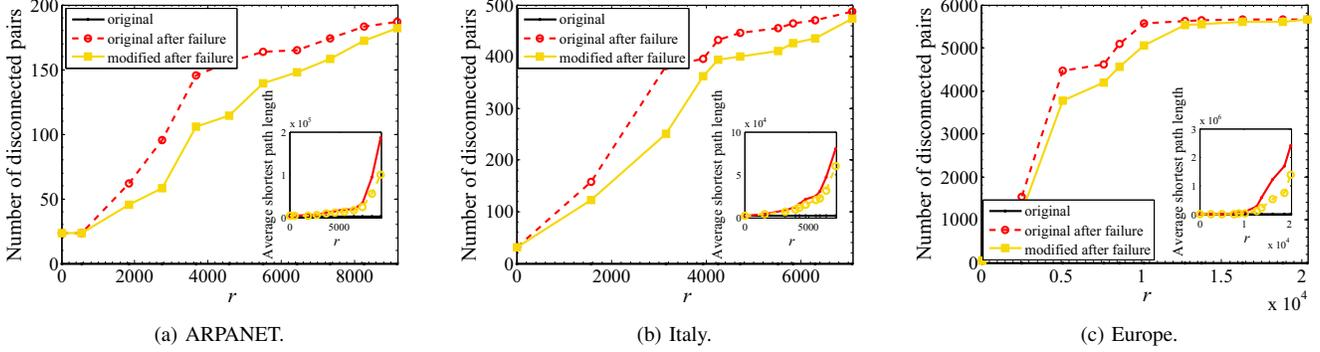
Fig. 10: The number of disconnected pairs and the average shortest path length (inset) as a function of the failure radius  $r$ . Ten links were added to each of the modified networks. The number of disconnected pairs in the original network is 0.
