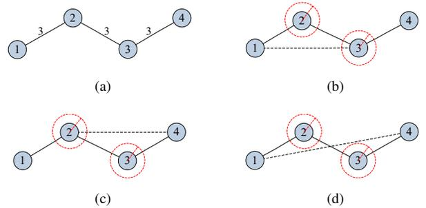
Fig. 4: Example of the network augmentation technique, with  $r = 1$ . (a) The original network. There are three possibilities for a link addition (shown in dotted lines). (b) Link (1, 3) is added. Critical region around 3 remains; (c) Link (2, 4) is added. Critical region around 2 remains; and (d) Link (1, 4) is added. Failure of any single critical region always leaves three connected pairs.
