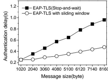
**Fig. 2.** Comparison of authentication delay between lock-step and sliding window protocols
