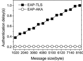
**Fig. 1.** Authentication delays of EAP-TLS and EAP-AKA with respect to the message size. EAP-AKA has a shorter delay because all messages in EAP-AKA fits to a single EAP message
