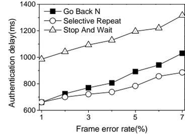
**Fig. 3.** Comparison of authentication delay between error recovery mechanisms with EAP message of 8160 bytes
