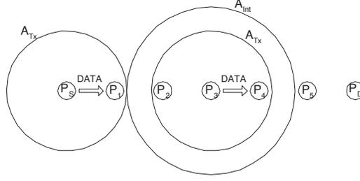
**Fig. 2.** Chain of 7 nodes separated by 200m from each neighbor. The interference range is according to Equation 1
