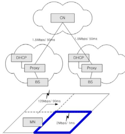
**Fig. 3.** Simulation Model
