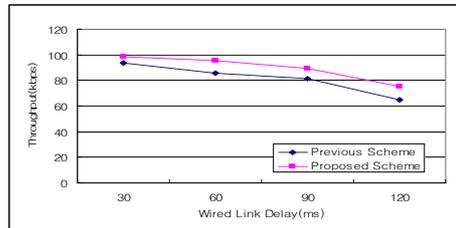
**Fig. 5.** Throughput according to wired link delay
