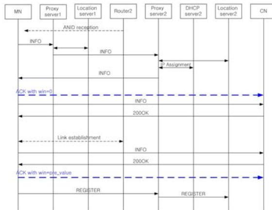
Fig. 2. Message flow in proposed scheme
