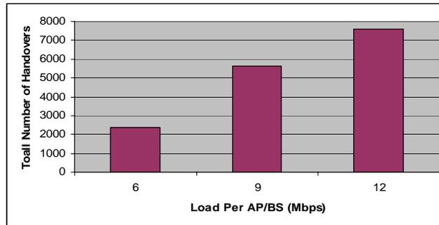
**Fig. 6:** Network Load Vs. Total number of handovers
