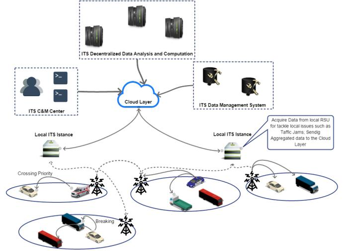
Fig. 1. The proposed multi-layered architecture used for improve road safety and reduce traffic jams.
