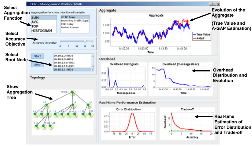
Figure 1. Interface on the management station for evaluating A-GAP on the testbed. It shows the effect of changing the accuracy objective from 0 to 15 flows, at time 14:42:30 in a testbed scenario. As a consequence, A-GAP reduces the overhead at the cost of an increased error in estimating the aggregate. The interface provides also real-time estimation of the error distribution and of the trade-off curve accuracy vs overhead.
