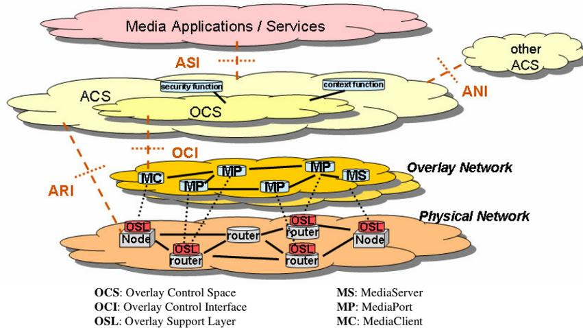
**Figure 1: The SMART SSON Architecture**
