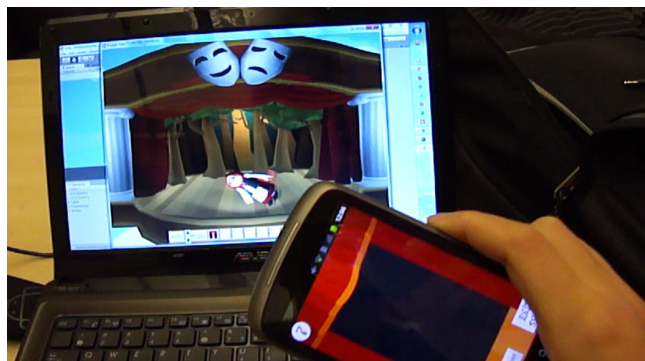
Fig. 3. Single phone control scheme; movements are directly projected onto the puppet body.
