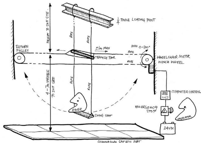
Figure 2 Illustration of mechanism of rope swing
