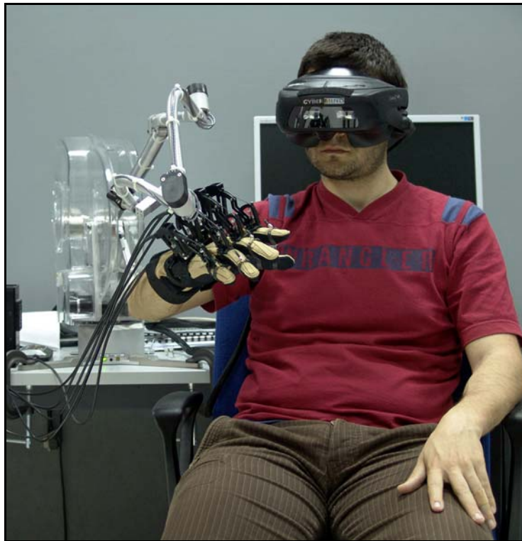
Figure 5 - Direct first-person hand interaction in the proposed virtual maintenance application using the CyberForce force feedback system.
