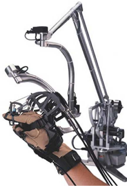
Figure 3 - The Immersion CyberForce articulated exoskeleton and the related CyberGrasp
