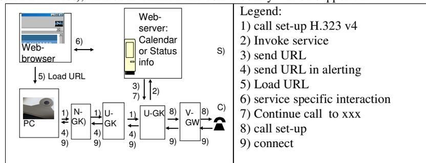
**Figure 5** Multimedia features in a Multi Media over IP system (based on Ericsson [22]). The entities are placed in accordance with Figure 3
