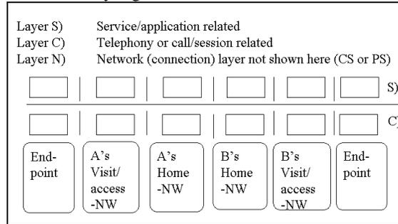
**Figure 3** Reference figure. Such a figure may be used to analyze business relations in a system. It can also be used to compare the architecture of GSM and IMS. (For more details, see [18])
