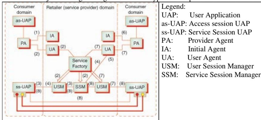
**Figure 6** TINA service session initiation with domains and multimedia streams shown. Figure from [12]. The numbers are referring to method invocations explained in TINA [3]
