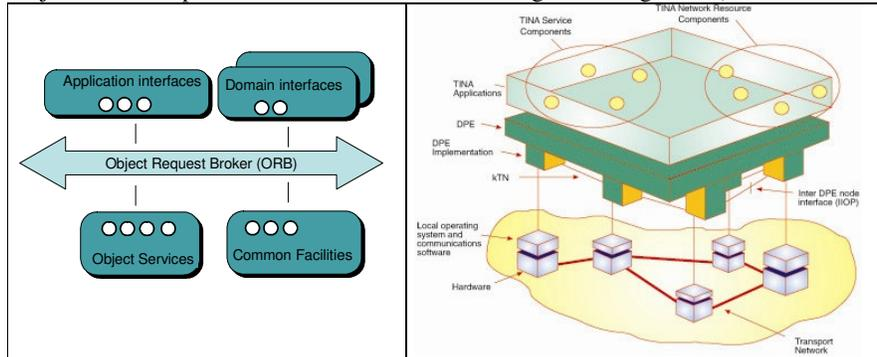
**Figure 2** Illustration of two different views of middleware. From a computer science view the network is often not shown (left). Quite naturally coming from the telecom side, TINA shows the networks: Transport Network (TN) and kernel TN (kTN). 2.1) Left: OMG-like from [12]. 2.2) Right: TINA-like, see e.g. [13]
