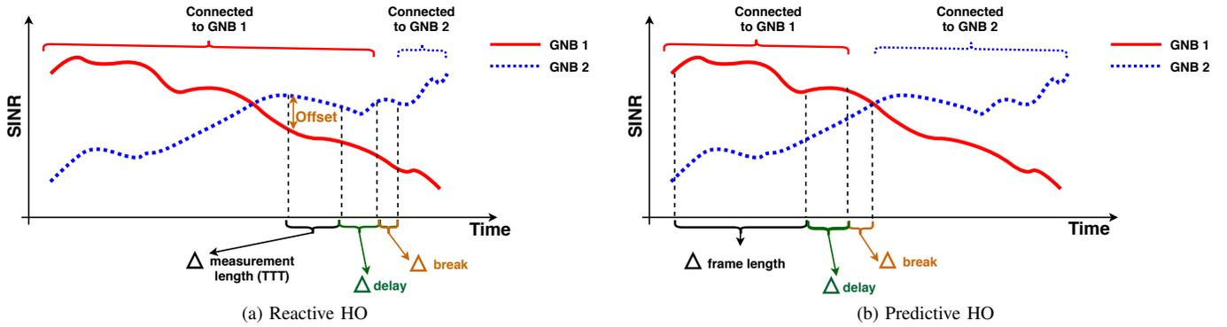
Fig. 1. Different HO mechanisms
