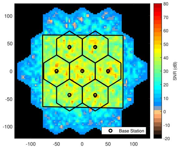
Fig. 3. Signal-to-Noise Ratio (SNR) map of the factory environment
