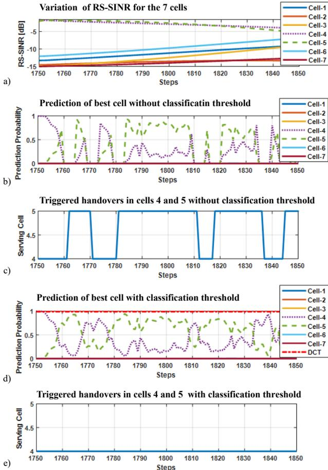
Fig. 4. prediction performance for a user along the edge of cells 4 and 5 without DCT
