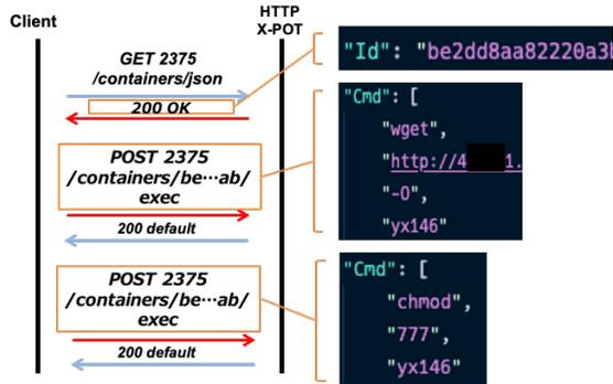
Fig. 3. Docker API Attack Flow (Observation Experiment).
