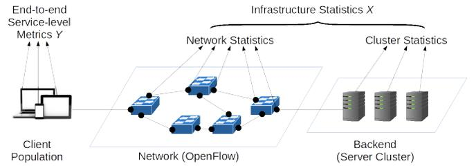
Fig. 2. Testbed used for experiments at KTH. In all scenarios KV and VoD performance metrics from infrastructure measurements are predicted [18]
