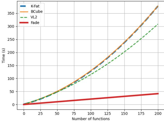
Figure 6. Evolution of the time required by each solution evaluated to obtain a valid configuration for VNs with different number of functions to be embedded onto the SN of the same size.
