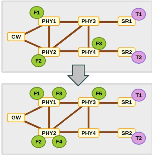
Figure 1. Illustrative example of the changes required to adapt a VN after deciding to add two new VNF instances and resolving the VNEP to get the best configuration. *GW* is the gateway, *PHY* are NSNs that instantiate functions, labeled as *F*, and *SR* nodes are high-end servers hosting resources, labeled as *T*.
