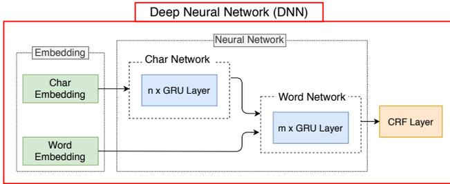
Fig. 2. Deep Neural Network (DNN) for sequence tagging
