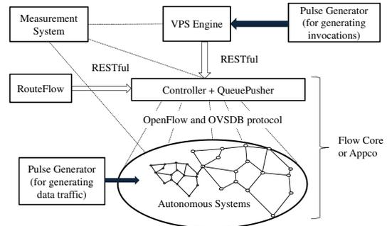
Fig. 2: CityFlow's architecture and components
