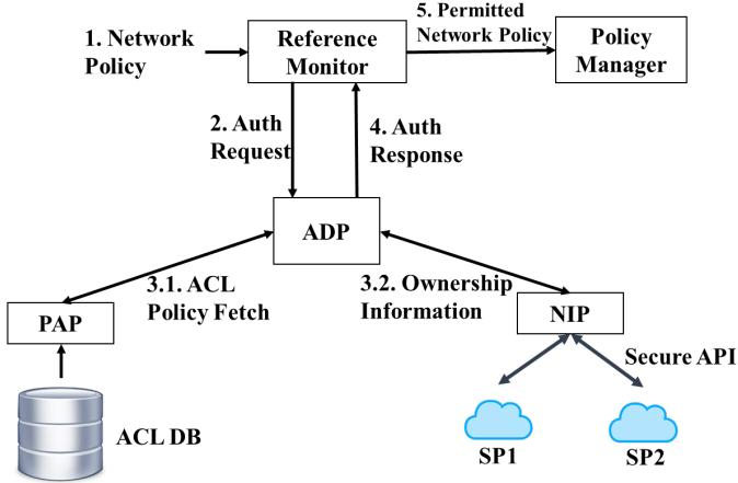
Fig. 6. Authorization process in the Reference Monitor Module
