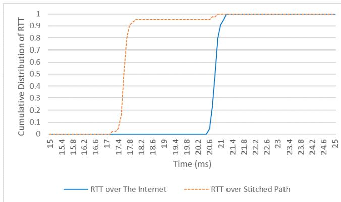
Fig. 9. RTT comparison of the regular path over the Internet vs the directed path through the exchange point
