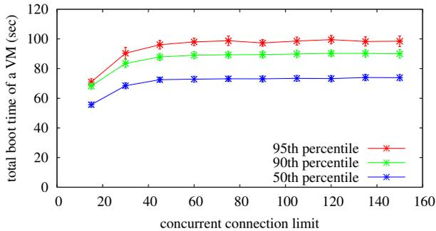
Fig. 8. Effect of the concurrent connection limit on total boot time of VMs in Cloud-B obtained from Rally
