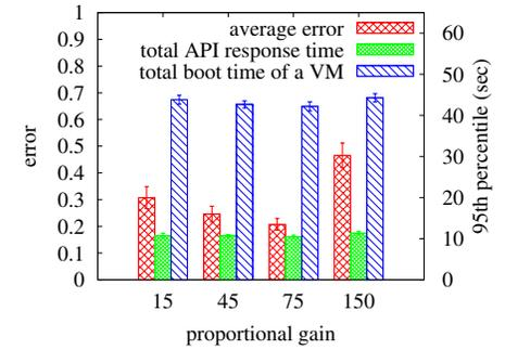
Fig. 12. Effects of the proportional gain in Cloud-A.
