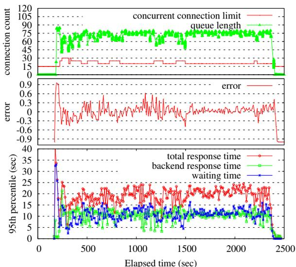
Fig. 10. Behavior of our adaptive limit controller and its effect in Cloud-B
