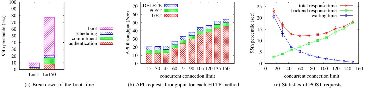
Fig. 5. Detailed effects of the concurrent connection limit in Cloud-A
