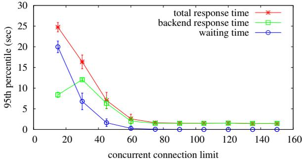
Fig. 6. Effect of the concurrent connection limit on API response times in Cloud-B obtained from HAProxy
