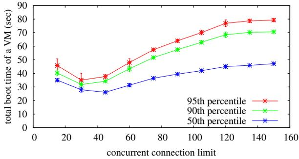
Fig. 4. Effect of the concurrent connection limit on the time to boot a VM in Cloud-A obtained from Rally
