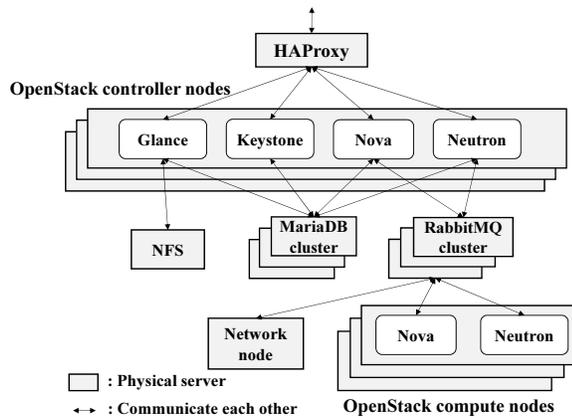
Fig. 1. OpenStack architecture and example of an OpenStack physical configuration. OpenStack controller nodes and individual components are configured to be redundant and scalable.
