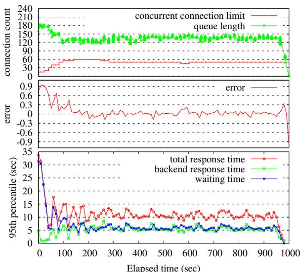
Fig. 9. Behavior of our adaptive limit controller and its effect in Cloud-A
