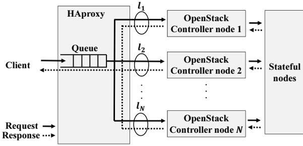
Fig. 2. Limiting concurrent connection on HAProxy
