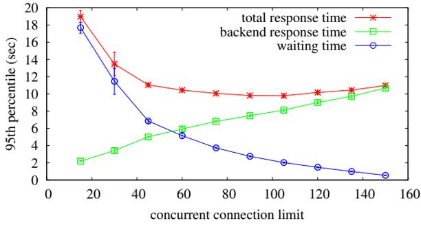
Fig. 3. Effect of the concurrent connection limit on API response times in Cloud-A obtained from HAProxy
