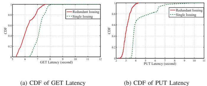
Fig. 2: Cumulative Density Function (CDF) of accessing 32 Mb data file in Amazon S3 with 3 replicas (redundant) issuing and no replicas (single) issuing.
