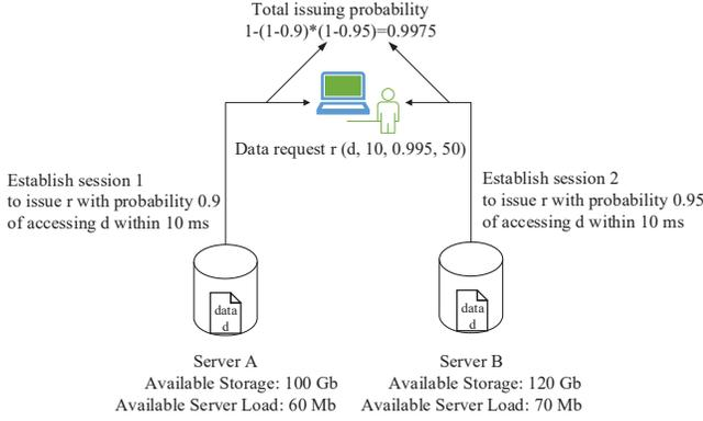
Fig. 3: Placing data on two servers using one session on each server to satisfy accessing data latency probability.
