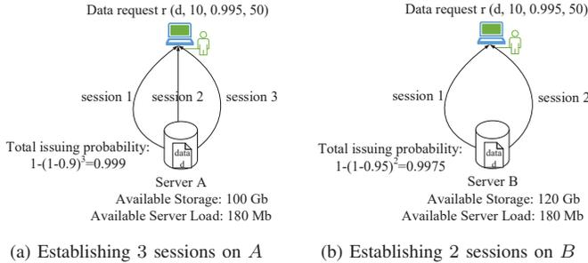
Fig. 4: Placing data on single server using multiple sessions to satisfy accessing data latency probability.
