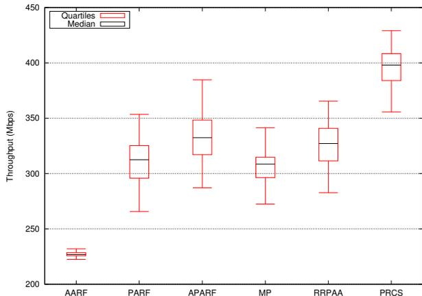
Fig. 6. Global Network Throughput in the High-Density Scenario.
