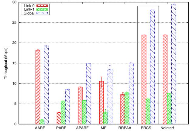
Fig. 4. Throughput in the Two-Links Scenario.
