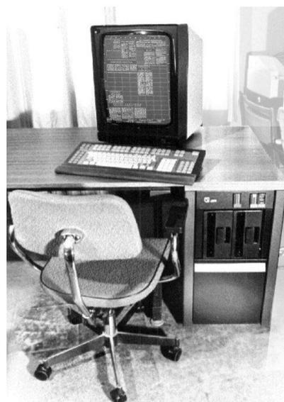
keyboard is set on a pull-out frame located underneath the desk surface and allowing configuring position and angles. The keyboard had 137 buttons, 134 of them fully pre-programmable; that is, a driver defines their layout and semantics.
