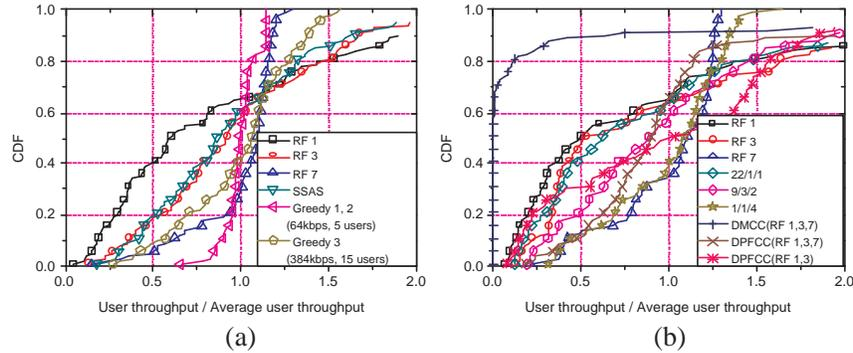
**Fig. 5.** (a) Fairness comparison of SSAS and the proposed schemes in flat fading; (b) Fairness comparison of proposed schemes in selective fading
