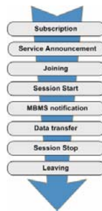
Fig. 2. Phases of MBMS multicast service provision
