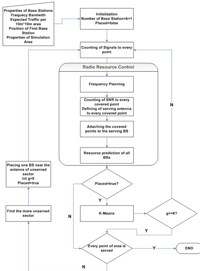
Fig. 4. Detailed flowchart diagram of RF planning algorithm
