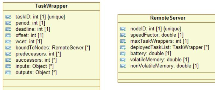
**Fig. 3. Characterization of the Remote Servers and Tasks**
