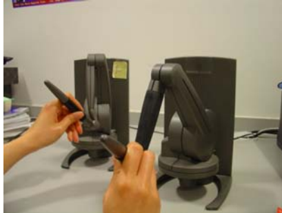
Fig. 1 PHANTOM Desktop Devices, Haptic Traffic Generation Devices
