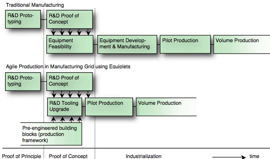
Figure 1: Concurrent development and engineering of High Volume manufacturing processes during the late proof of concept phase. By upgrading well-chosen production technology from R&D to production, a significant time gain can be achieved in bringing new developments to the market.
