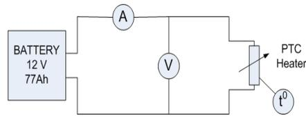
**Fig. 6.** Measurement scheme for determining  $U = f(I)$  characteristics.
