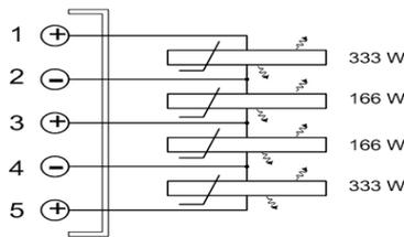
**Fig. 7.** Electrical diagram of the PTC heater sample.
