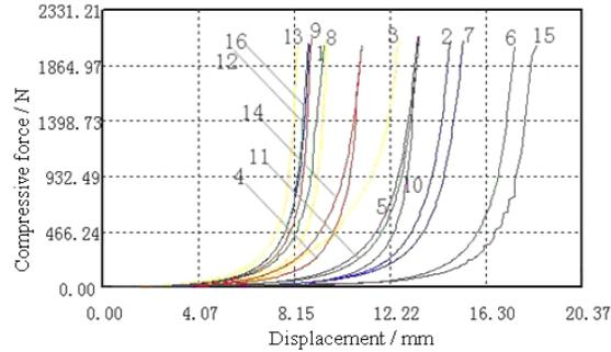
**Fig. 3.** Compression curves of fish floss with different processing methods
