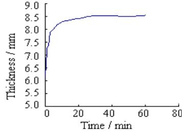
Fig. 2. Relaxation characteristic curve of molding block
