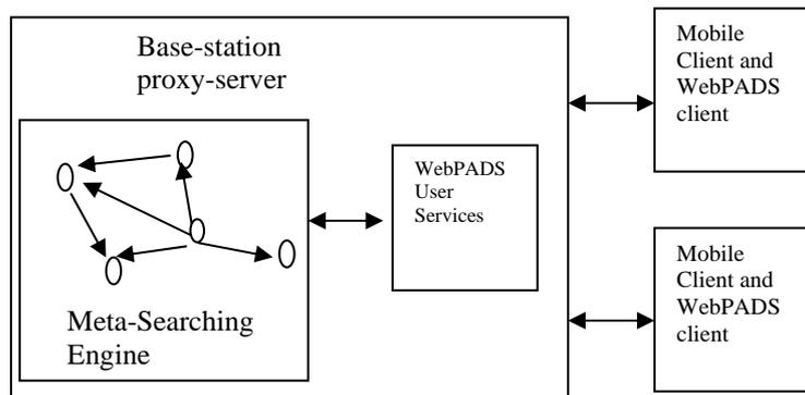
Fig. 2. System Architecture
