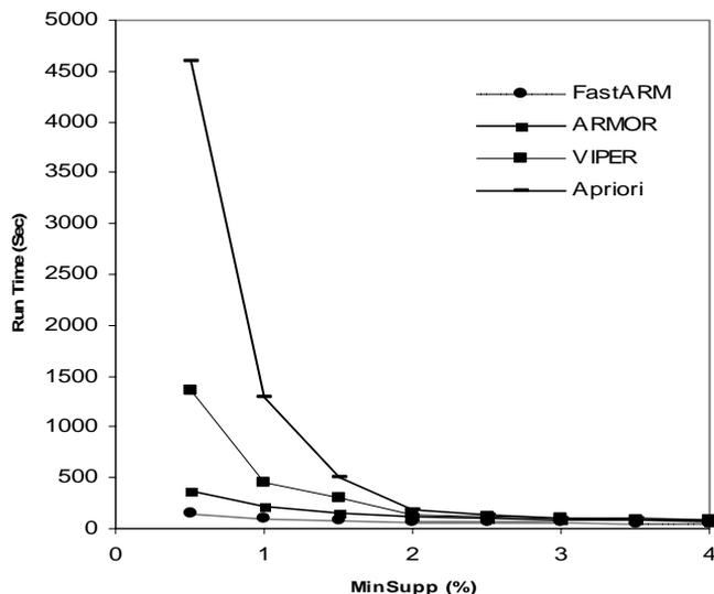
Fig. 3. Performance of different methods on synthetic data for different Minsupp values
