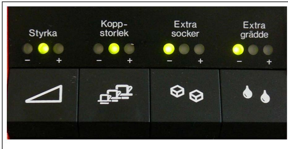
**Fig. 3.** The adjustment buttons on a common coffee vending machine in Sweden. The labels on top read 'Strength', 'Cup Size', 'Extra Sugar' and 'Extra Cream' from the left to the right. The question is what the minus signs signify in combination with the expression 'Extra...'
