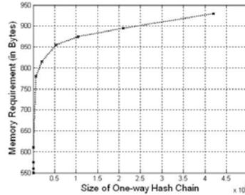
Fig. 4. Memory requirement for One-way Hash Chain generation
