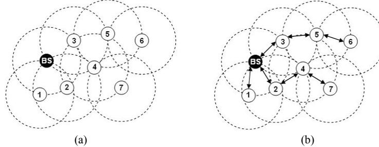
**Fig. 1.** (a) Network in the initial state (b) After initialization phase is over. Here, we have three paths,  $B \rightarrow 3 \rightarrow 5 \rightarrow 6$ ,  $B \rightarrow 2 \rightarrow 4 \rightarrow 7$  and  $B \rightarrow 1$  along which the one-way hash chain number is initialized. The dashed circles indicate the transmission ranges of the nodes.
