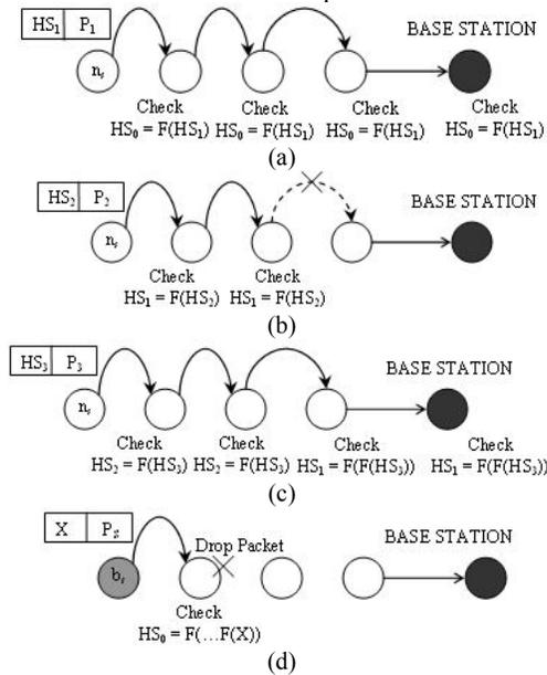
**Fig. 2.** (a) Authenticated packet delivery to BS (b) A packet could not reach the BS (c) OHC verification method is not hampered (d) Bogus packet detection and dropping
