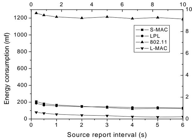
Fig.6. Energy consumption under different source report interval
