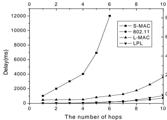
**Fig.3.** Mean packet latency on each hop under low traffic load
