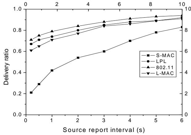
Fig.7. Throughput under different source report interval
