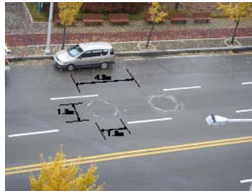
Fig.2. Loop detectors at the field test site
