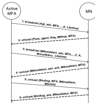
Fig.2. Passive agent election and binding signaling.
