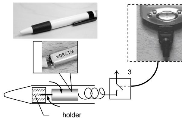
Fig. 1. Vibro-tactile pen: general view and schematics.
