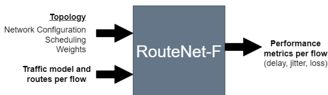
Fig. 2: Inputs and outputs of RouteNet-F. [4]
