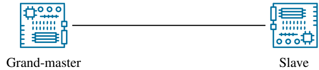
Fig. 7: Network setup for n = 0 , direct measurements – the difference meter is not included in these diagrams as it's not connected to any device via Ethernet
