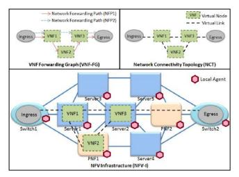
Fig. 1: Mapping of the VNF-FG in the NFV-I.
