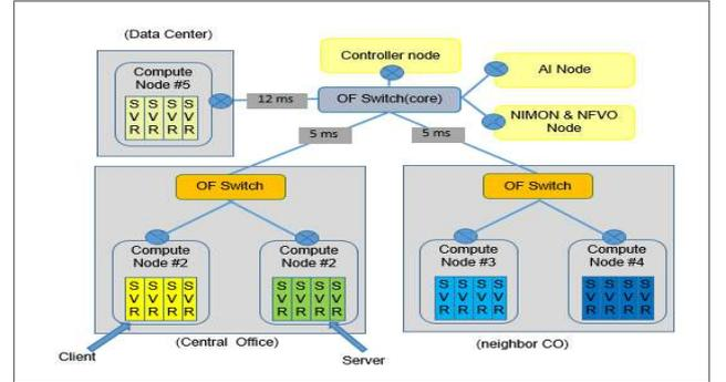
Figure 1. Physical Infrastructure with OpenStack Management Layer
